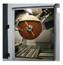
The Side Door provides the user easy access for cut off wheel changes
