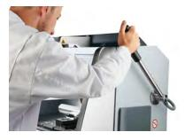
The integrated hand lever comes equipped with **EasyLock** to regulate cutting force and achieve greater precision. Push button operation allows operator to easily set the vertical position for automatic horizontal cutting (X-cut)
