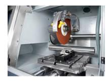
A no-drip **sliding front door** and swinging side door allow optimal access to the working area, which features LED lighting and a safety interlock
