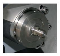
The **EasyNut** is a simple device that locks tight on the arbor shaft yet can be easily removed by anyone in the lab for fast wheel changes. The **Quick Change System** is a removable and easily replaceable arbor that reduces maintenance costs
