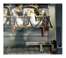
The **Automatic Cross Feed** enables horizontal movement of the cutting wheel to achieve precision Z-axis serial cuts
