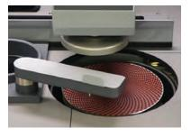
Programmable **Dosing Arm** ensures repeatability for multi-step processes using diamond suspensions, lubricants and oxide
