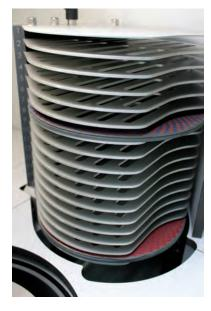
16 place **Media Elevator** quickly sorts and exchanges grinding/polishing media
