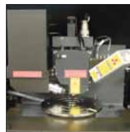
Soft X-ray Charge Neutralizer (X-ray leakage protective cover attached)
