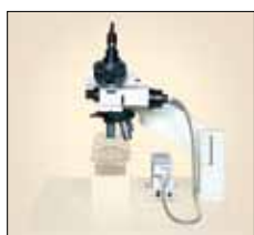
Objective lens \times 5 , \times 20 , \times 50 With differential interference function Monitor magnification: 2800 (on a 19 inch monitor)
