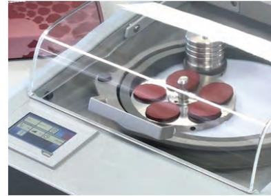
If left unattended, the **Surface Guard** feature periodically vibrates after program completion, minimizing corrosion and/or crystallization of the sample surface
