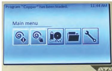
Touch screen control panel includes pre-installed preparation methods, an option for automatic frequency control and up to 200 user programs
