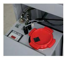
Optional **Recirculation Coolant System** maintains constant water temperature with refrigeration coils
